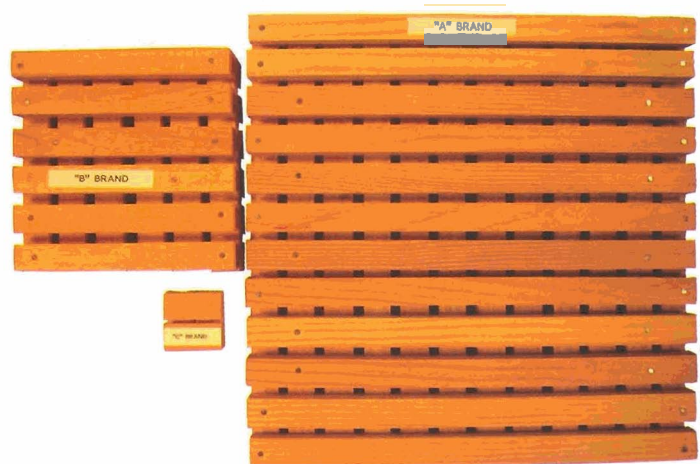
The Class A and B brands consist of a three-layer sandwich of 3/4” square sticks that are nailed together. The Class C brand is much smaller, consisting of an individual piece of wood about the size of an ice cube.
