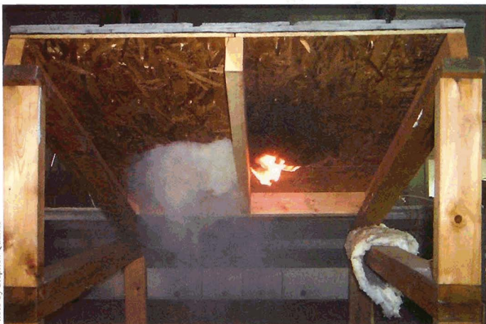
Flame penetration occurred on the bottom of this deck, therefore, the roof covering failed to meet the requirements for a Class A rating. Flame through occurred at a sheathing joint between two panels.
