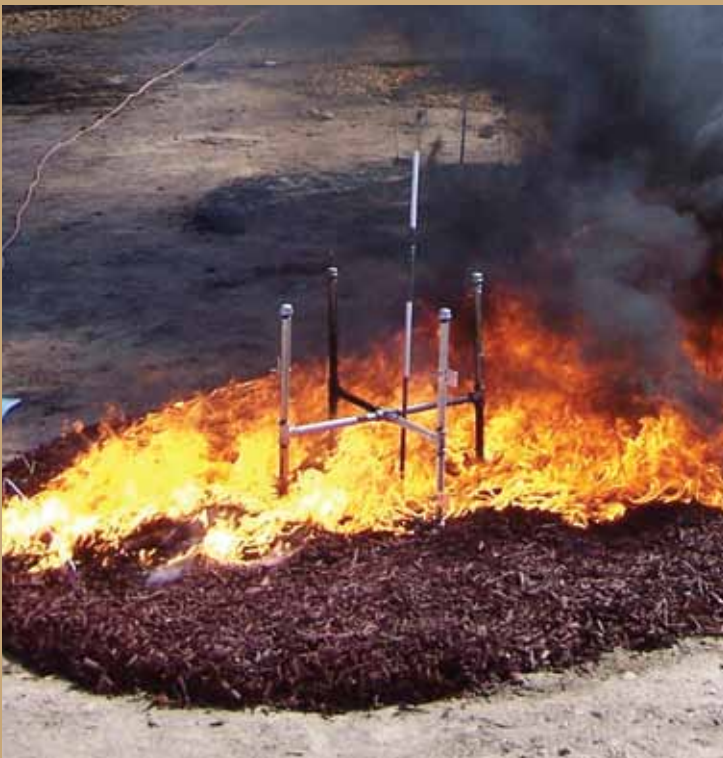
▲ Figure 4. Rubber mulch produced the greatest flame height and temperature of the mulch treatments evaluated in this study.
