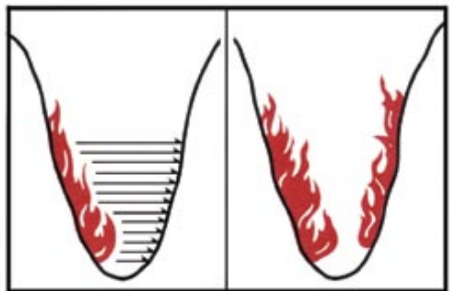
Flashover in V-shaped valley.
