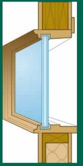
Figure 5-12: Thermopane window
