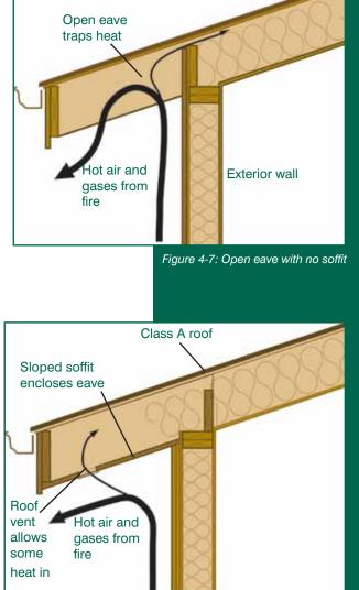
The eave should be covered with a soffit. If the soffit is applied directly to the rafter eave, it forms a sloping soffit, which creates a pocket that can trap fire.
