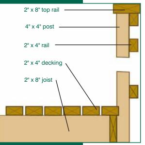
Decks are built to burn almost as easily as wood stacked in a fireplace. All the components of a deck – joists, decking and railings – generally are made of wood, plastic or wood-plastic composites generally no more than 2 inches thick with high surface-to-volume ratios.
