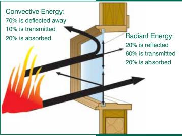
Figure 5-10: Energy transmission, conventional glass
