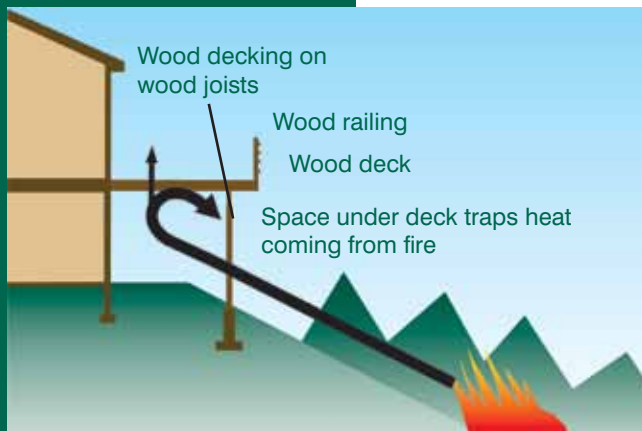
Figure 4-10: Conventional deck in a fire
