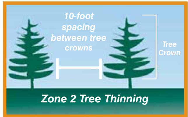
Figure 17: In Zone 2, make sure there is at least a 10-foot spacing between tree crowns. Credit: CSFS
