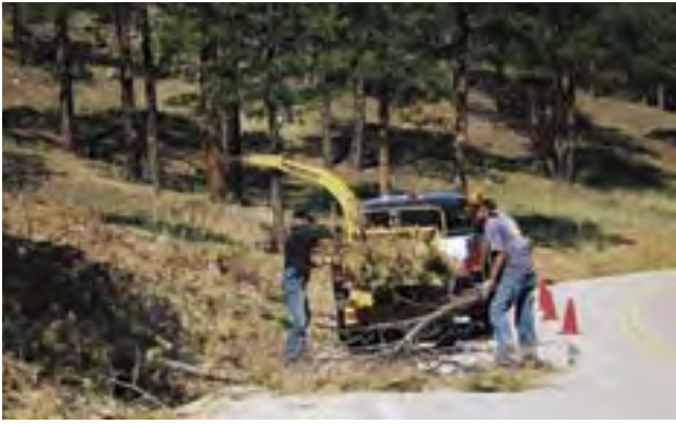
Chipping is the most desirable, but also the most expensive method of slash disposal.
