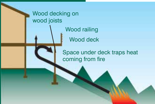
Figure 4-10: Conventional deck in a fire
