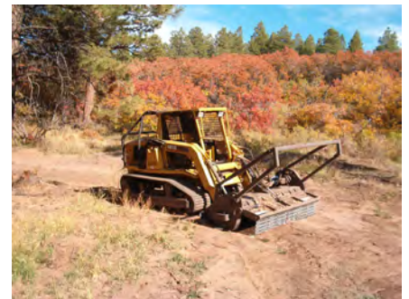
Figure 4. Mechanical treatment using a timberaxe.
