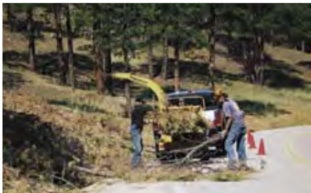
Chipping is the most desirable, but also the most expensive method of slash disposal.
