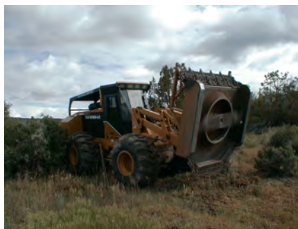
Figure 3. Mechanical treatment using a Hydroaxe®.
