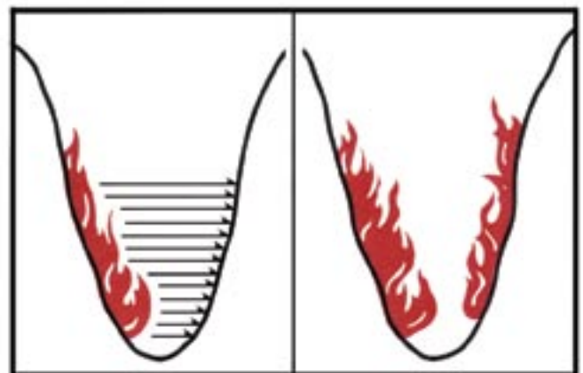
Flashover in V-shaped valley.
