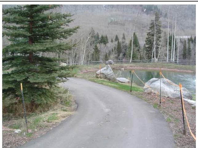
Driveway is very narrow here- limb up or (preferably) remove conifer, and widen drivable surface, or make sure soils are compacted so fire trucks don't get stuck in soft soils.
