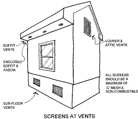
**Attic, Subfloor or Foundation Vents:** Wind and/or direct contact with a fire’s convective heat can push firebrands through the vents into your home’s basement or crawl space.
