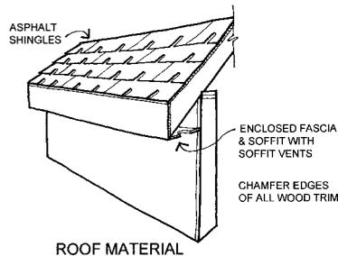
The best way to avoid this situation is to make sure your roof is fire-resistant. The two main fire resistance tests used today include: ASTM E108 and UL 790. There are three levels of classification awarded under the test protocol, A, B, and C, with A being the most
