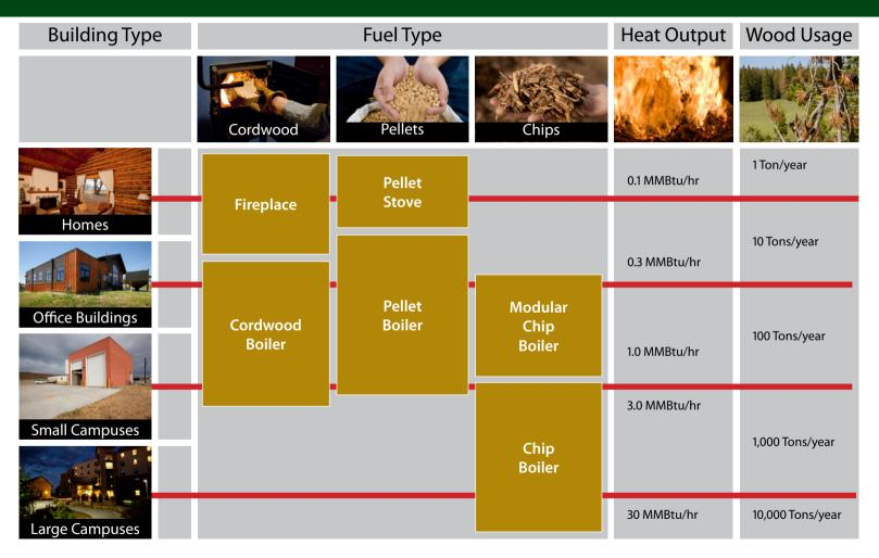
This chart provides a rough idea about which technology makes sense for various application. It is not a planning or design tool.
