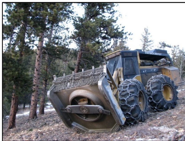
Figure 2. Hydroaxe used for mastication of heavy woody fuels.
