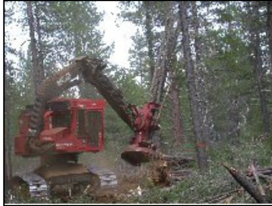
Figure 7. A feller buncher machine thinning a forest. Photo from USFS.
