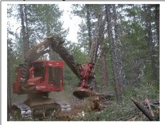
Figure 6. A feller buncher machine thinning a forest. Photo from USFS.
